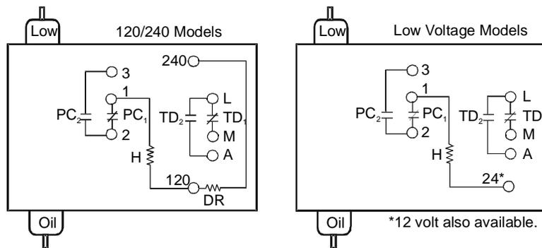
PC<sub>1</sub> - Pressure actuated contacts. Open on increase in pressure difference between oil and low pressure connectors. Makes and breaks time delay heater circuit.
