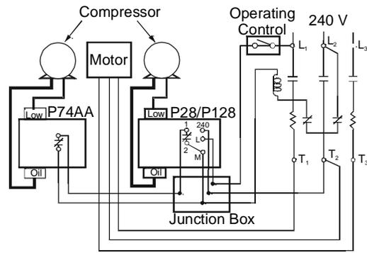
Note: This system would provide shutdown on low lube oil pressure in either of two compressors operated by the common motor.
