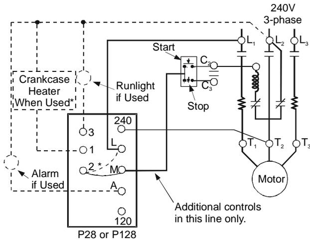
\*When crankspace heater is used, disconnect jumper from 2 to M and reconnect 2 to L.
