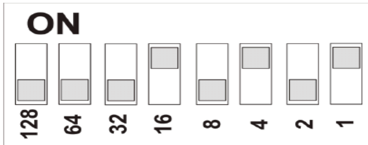
Figure 5: Setting the Device Address and Wireless Operation Mode on the MAC Address DIP Switch Block
