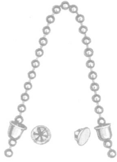
Fig. 2 -- Beaded chain with sleeves installed. The “snap” plugs are used to hold the chain in the thermostat.
